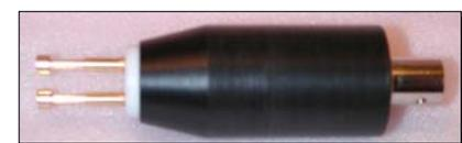
**Model 845:** A 1 lb (0.45kg) version of the ESDA STM4.1, ASTM F150 and NFPA 99 5 lb (2.2kg) Probe with a 2.5" (64mm) diameter conductive rubber electrode. Metal plate contact resistance is less than 100 Ohms when measured at 10V.
