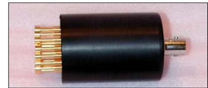
**Model 844:** A 2-Point Probe with two 0.125" (3mm) diameter conductive rubber electrodes spaced 0.25" (6mm) between centers. Minimum measurement size is 0.75" x 0.188" (19 x 5mm) with a 0.438" (11mm) cavity.
