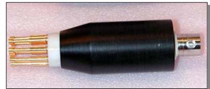
**Model 842:** A 1.5" (38mm) diameter concentric ring Probe with an inner ring of five 0.062" (1.5mm) electrodes and an outer ring of seventeen 0.156" (4mm) diameter electrodes on 0.875" (22mm) centers. Minimum measurement size is 1.25" (32mm) and a 0.25" (64mm) deep cavity.
