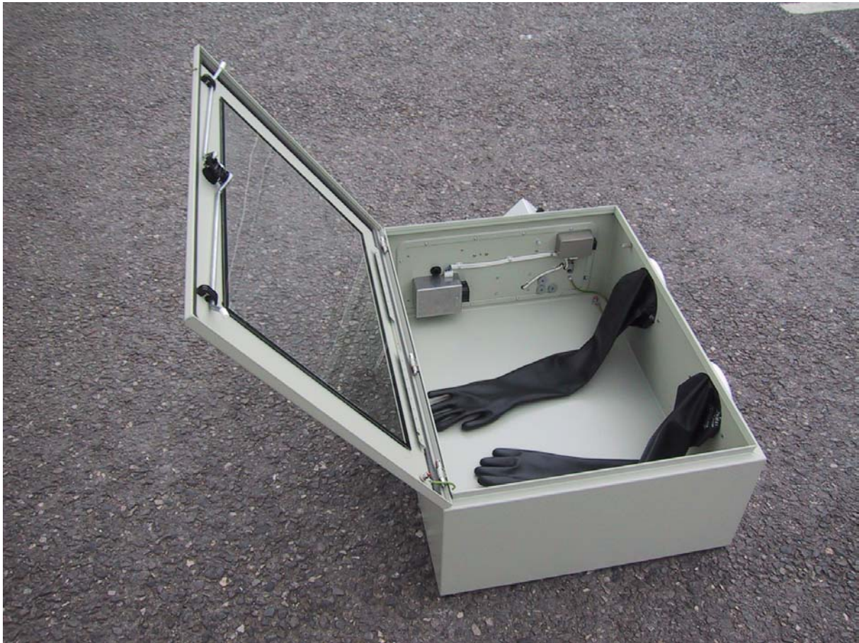
Inside of JCI 191 Controlled Humidity Test Chamber
