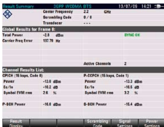
Analyse eines 3GPP WCDMA-Sendesignals.
