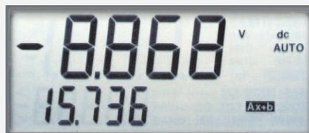
This means, for example, that the electrical output of a transducer can be scaled to give a direct readout of the physical parameter e.g. temperature or weight. It is particularly useful with 4-20mA current loops.
