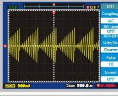
AM Modulation used by sine WAVE
